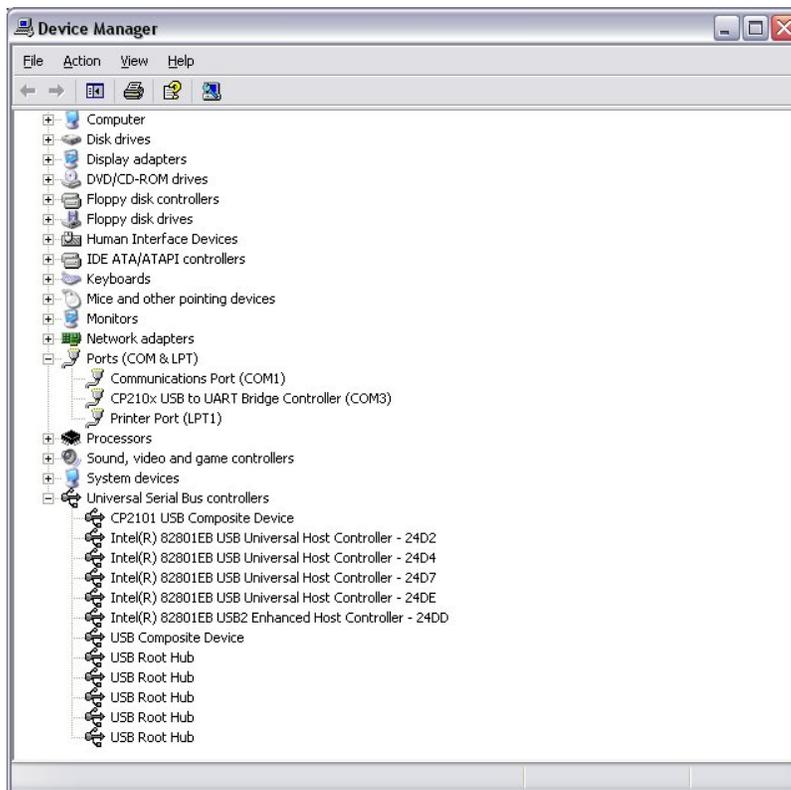
In the example above, a COM3 virtual serial port has been created. Note that the PC does not physically have a serial port 3, but one has been emulated by loading the appropriate USB driver ( in this case a CP210x bridge controller ).
