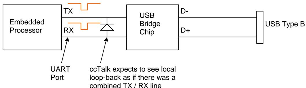
When the USB lead is plugged into the host PC, the application software in the PC will configure the baud rate in the USB Bridge Chip using the VCOM driver so that the embedded processor can operate as if the USB link was not present.
